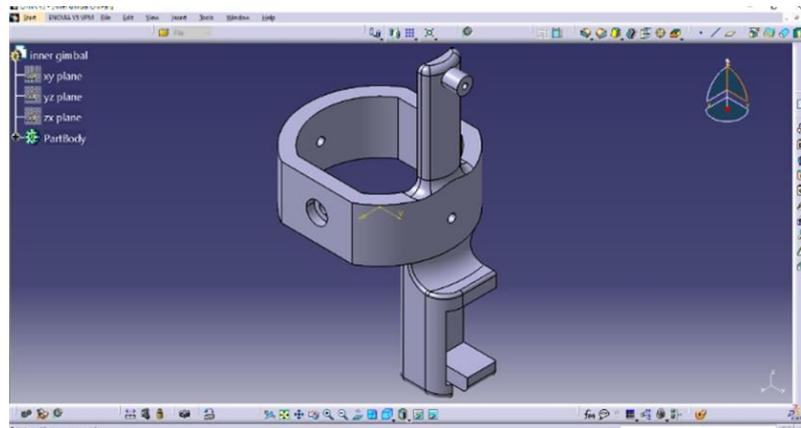
Fig. 3. CAD model of Inner Gimbal
