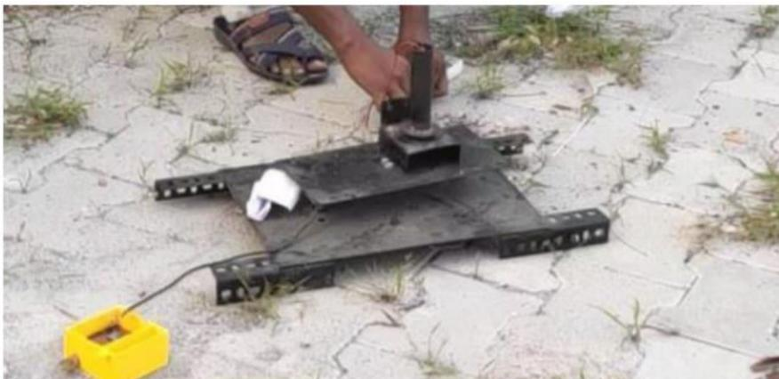
Fig 9. Thrust stand calibration
