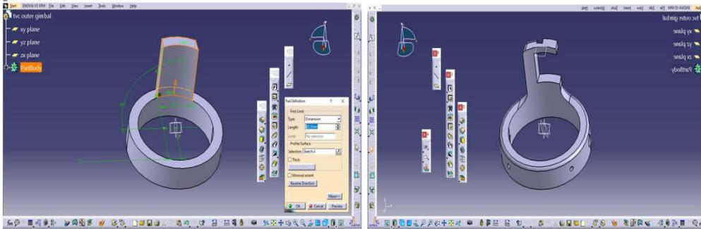
Fig. 2. CAD model of Outer Gimbal
