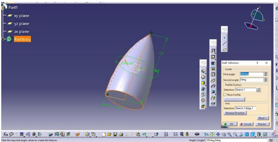
**Fig.6 CAD model of Nose Cone**
